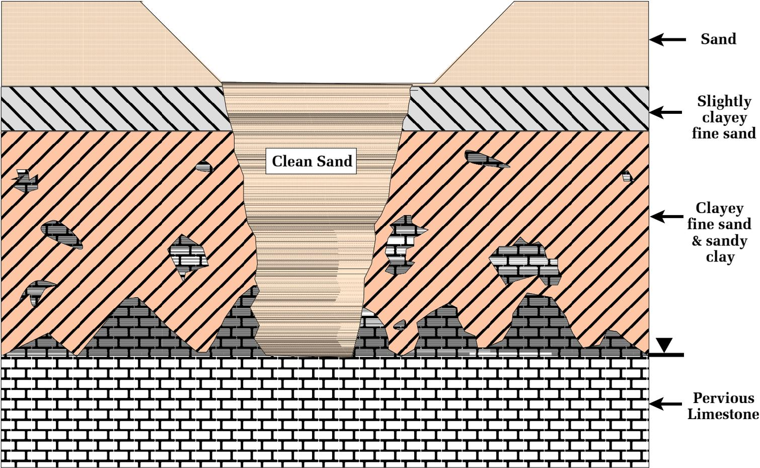
**RETROFIT OPTION #2 - OVEREXCAVATE & BACKFILL WITH PERMEABLE SAND**
