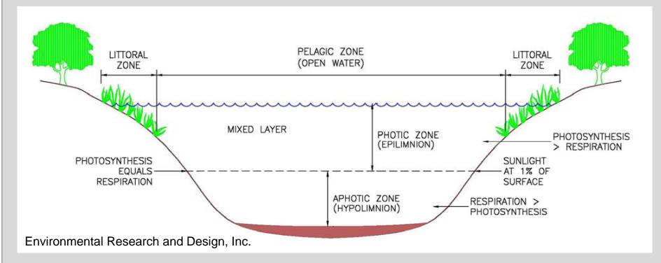
The volume of water below the anoxic depth does not provide treatment. Only the volume of water above the anoxic depth is used when calculating the permanent pool volume.
