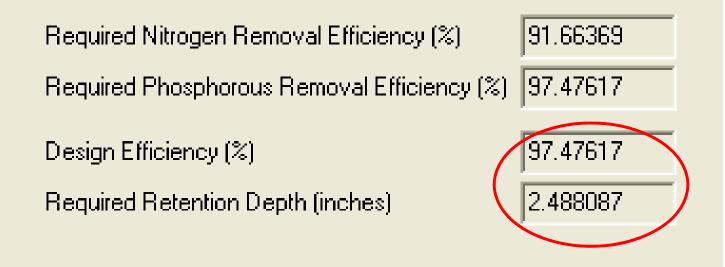
In an average year, the pond must retain and infiltrate 97.5% of the total runoff from the site.
