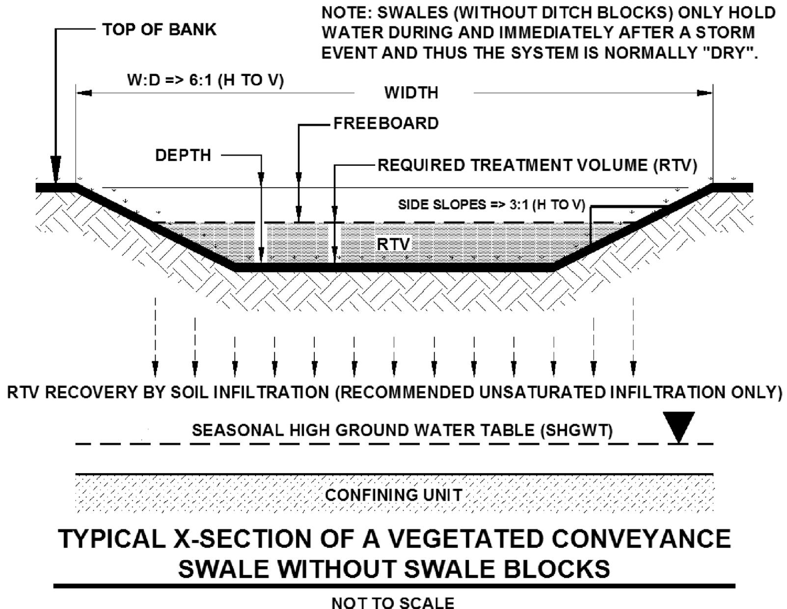
TYPICAL X-SECTION OF A MAN MADE DRY SWALE - AS OF 12-07-09.DWG
