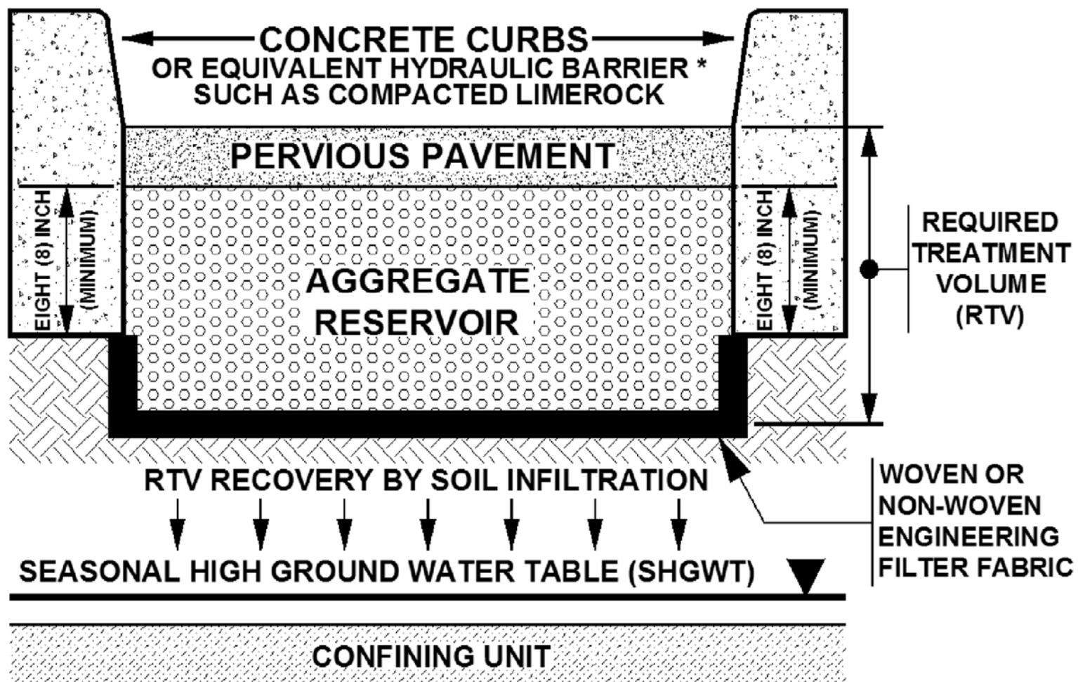
\* THE PURPOSE OF THE PERIMETER CONCRETE CURBING (OR EQUIVALENT BARRIER) IS TWOFOLD. FIRST, CONCRETE CURBING (IF UTILIZED) CAN ALLOW NUISANCE PONDING ABOVE THE PERVIOUS PAVEMENT. SECOND, CONCRETE CURBING WILL REDUCE HORIZONTAL SCOUR EROSION SHOULD THE SYSTEM FAIL.
