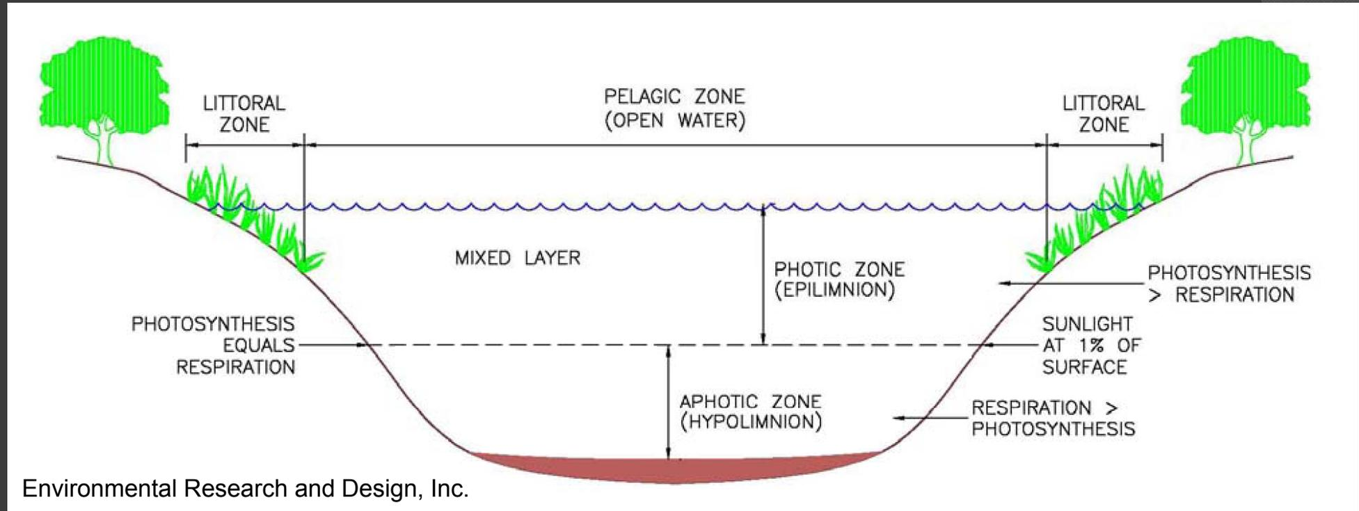
The volume of water below the anoxic depth does not provide treatment. Only the volume of water above the anoxic depth is used when calculating the permanent pool volume.
