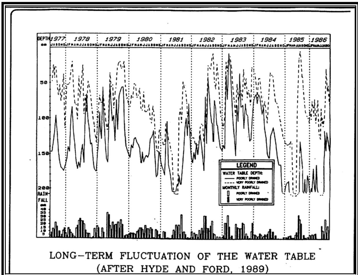
Figure 2. Recorded Long-Term Water Table Fluctuation
