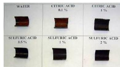
**Figure 4.** Treatment of iron scale formed within irrigation tubing with sulfuric acid, citric acid, and a proprietary product at selected concentrations. Iron scale on the inside of the tubing is evident by the reddish brown/rust color.
