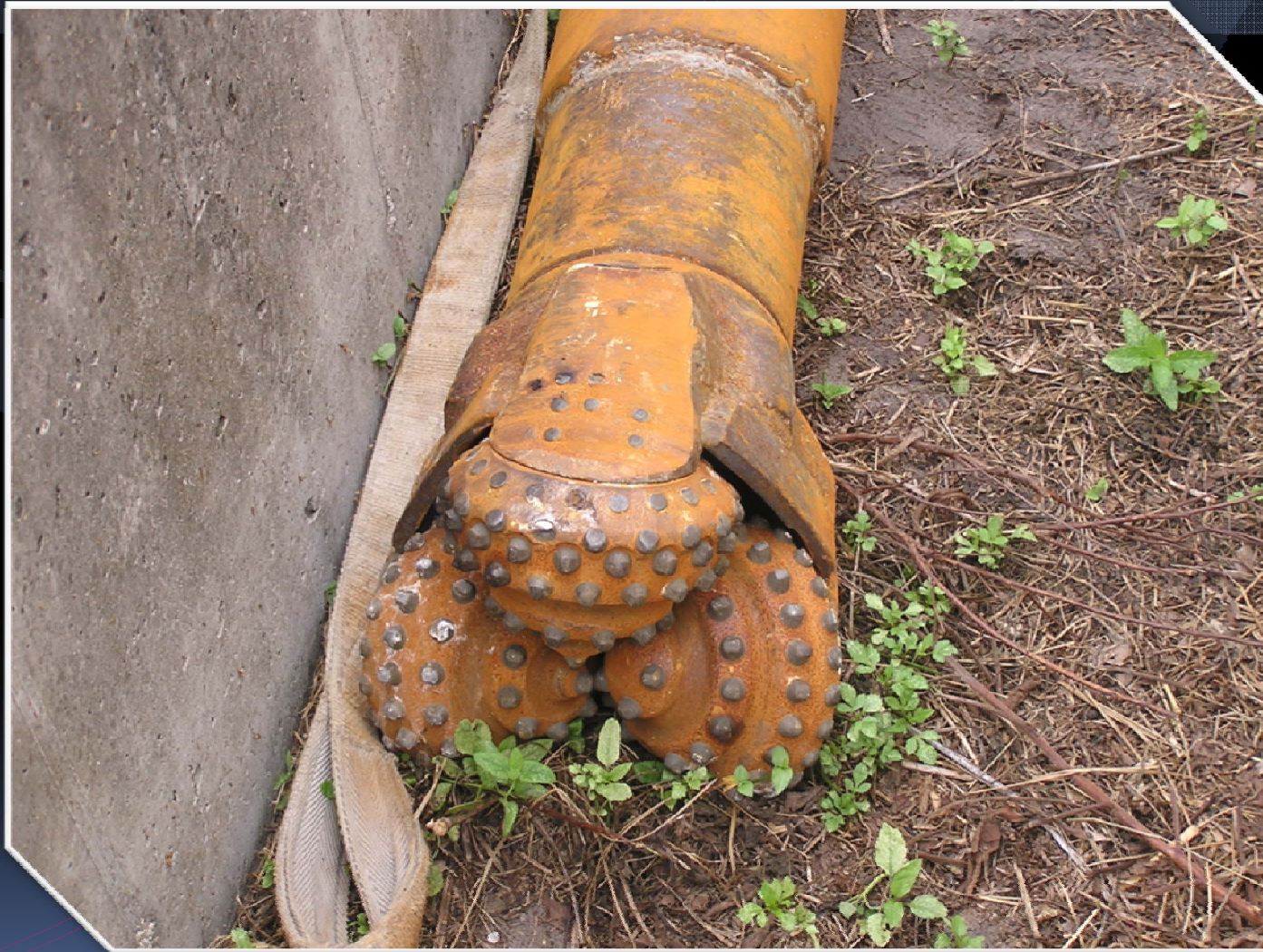
Bass Lake - Closeup view of 12-inch diameter drill bit.
