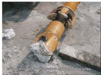
3-View of 16-inch diameter drill bit used to drill borehole below surface casing in order to set 10-inch well casing
