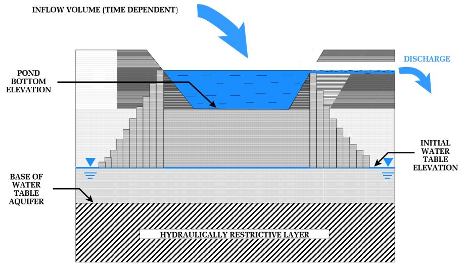
note: initial flat water table assumption is not unrealistic when the natural gradient is considered together with the duration of loading and the corresponding radius of influence.
