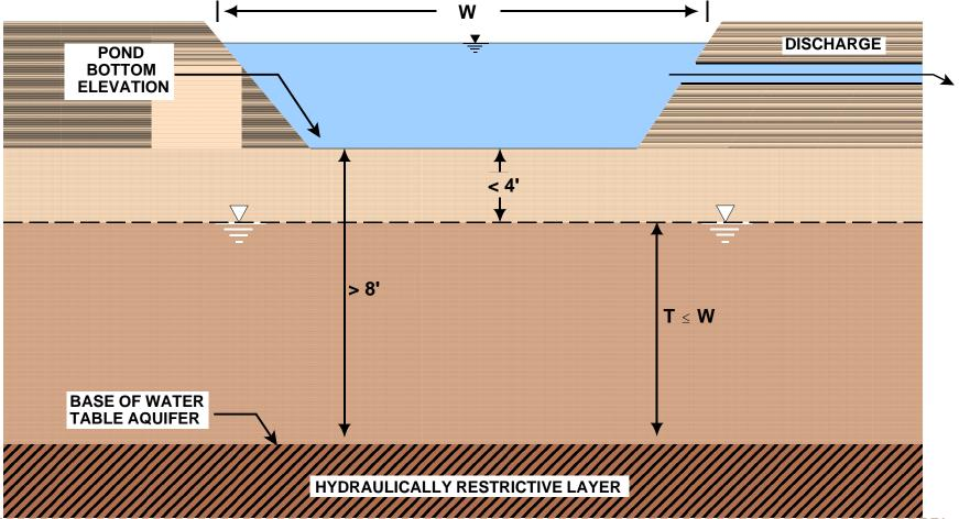
Model #2 - Dry Retention With Thick Aquifer & Shallow Water Table
