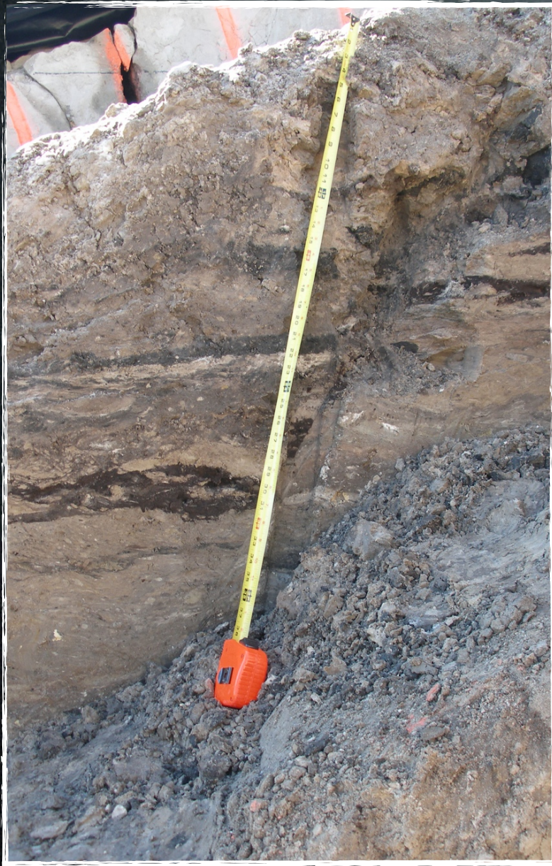
Close-up view of the shear failure plane on the southern pit wall
