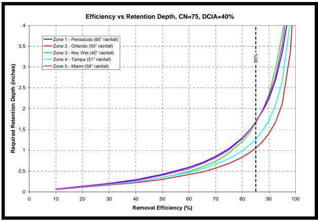
Exhibit 1.2. Efficiency vs Retention Depth at Several Locations for CN=75 & DCIA=40%
