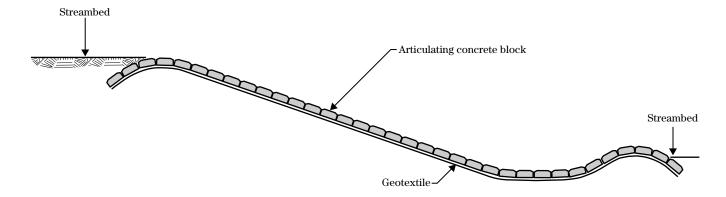
Figure TS14L-5 Armoring of pipe/culvert outlets profile
