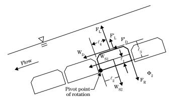
Figure TS14L-14 Forces on a protruding block (Figure courtesy of HCFCD)
