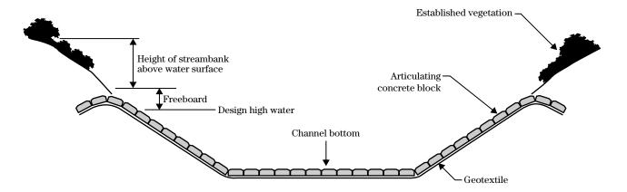
$\label{eq:Figure TS14L-2} \textbf{ Armoring the toe and lower slope cross section}$
