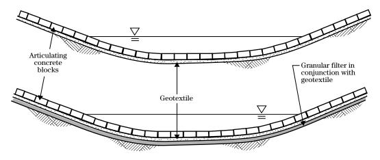
Figure TS14L-11 ACBs in combination with granular and geotextile filter
