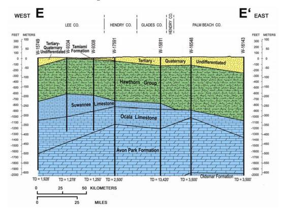
Figure 8. Cross section E-E'.
