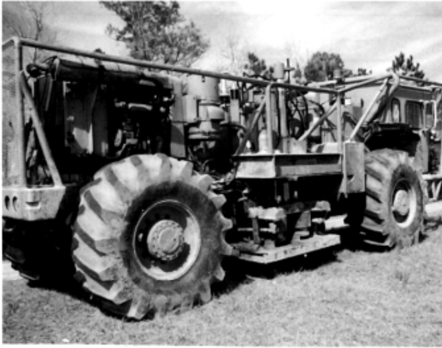
A "thumper," or vibroseis truck, produces environmentally safe seismic waves for oil exploration by pounding the ground with the large plate in the center. FGS photograph.
