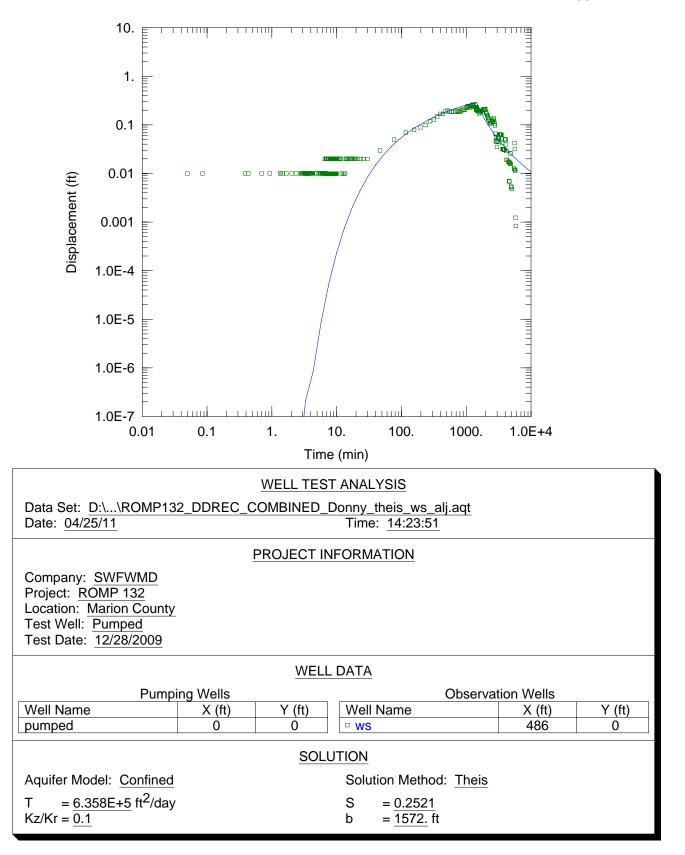
**Figure H-4.** Curve match solution output from AQTESOLV<sup>®</sup> using the Theis/Hantush method for the estimation of transmissivity (T) using groundwater level data collected from the water supply well during the Upper Floridan aquifer performance test at the ROMP 132 well site in Marion County.
