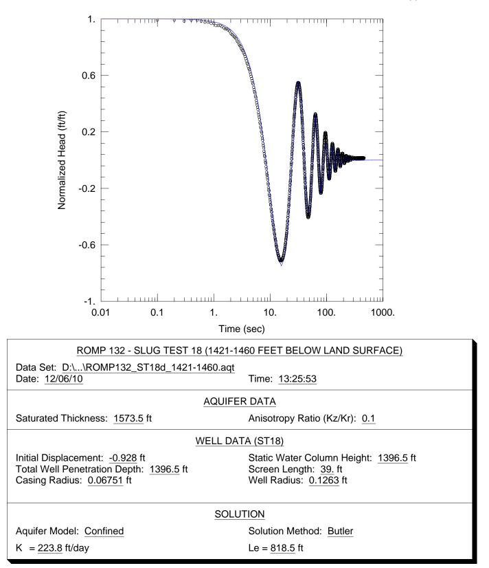
**Figure F-18.** Curve match solution from AQTESOLV<sup>®</sup> for hydraulic conductivity (K) using data from the slug test conducted between 1,421 and 1,460 feet below land surface (slug test 18) at the ROMP 132 well site in Marion County.
