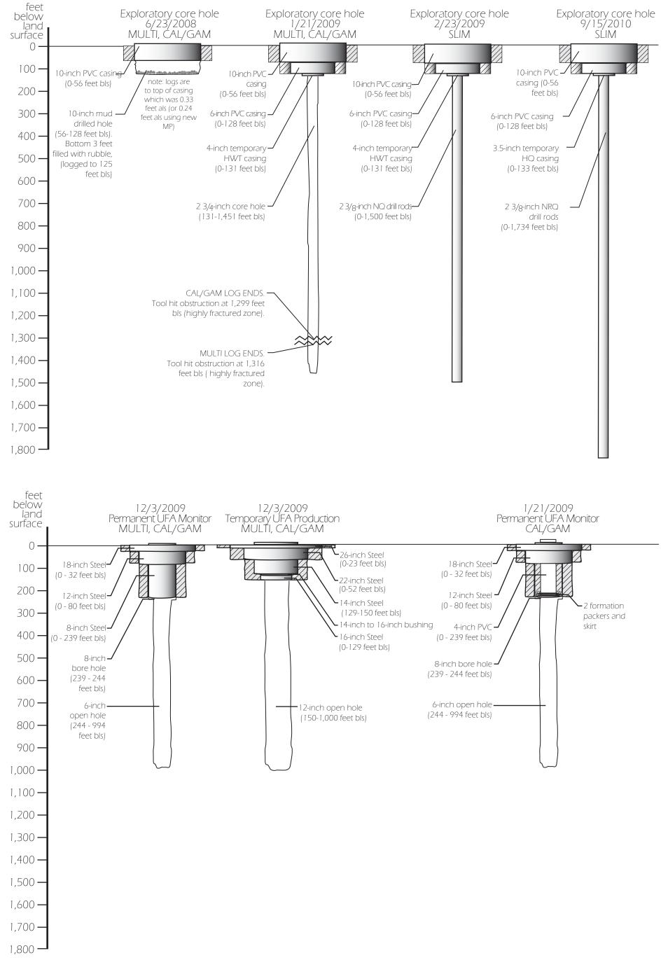
[Logs are to land surface unless otherwise noted; bls, below land surface; PVC, polyvinyl chloride; als, above land surface; MP, measuring point; ft, feet; HWT, temporary 4-inch steel casing; NQ, 2 3/8-inch steel drill rods; HQ, 3.5-inch temporary steel casing; NRQ, 2 3/8-inch steel drill rods; MULTI, multi -probe; CAL, caliper; GAM, gamma; SLIM, slim-line probe; UFA, Upper Floridan aquifer]
