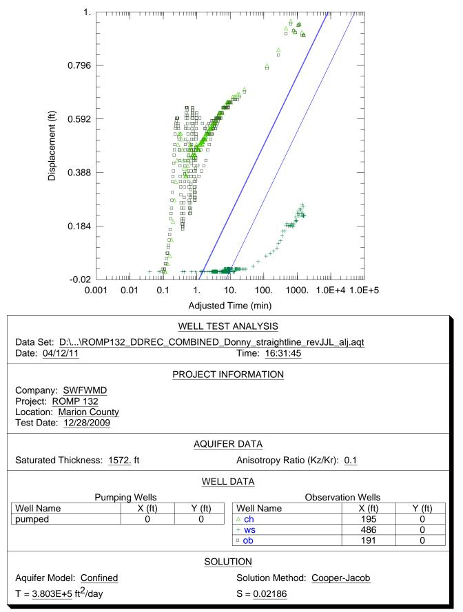
**Figure H-1.** Curve match solution output from AQTESOLV<sup>®</sup> using the Cooper Jacob straight line method for the estimation of transmissivity (T) using groundwater level data collected from the Upper Floridan aquifer monitor well, exploratory core hole, and drilling water supply well during the Upper Floridan aquifer performance test at the ROMP 132 well site in Marion County.
