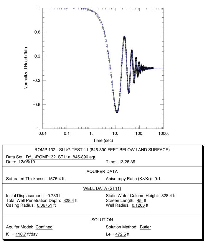
**Figure F-11.** Curve match solution from AQTESOLV<sup>®</sup> for hydraulic conductivity (K) using data from the slug test conducted between 845 and 890 feet below land surface (slug test 11) at the ROMP 132 well site in Marion County.
