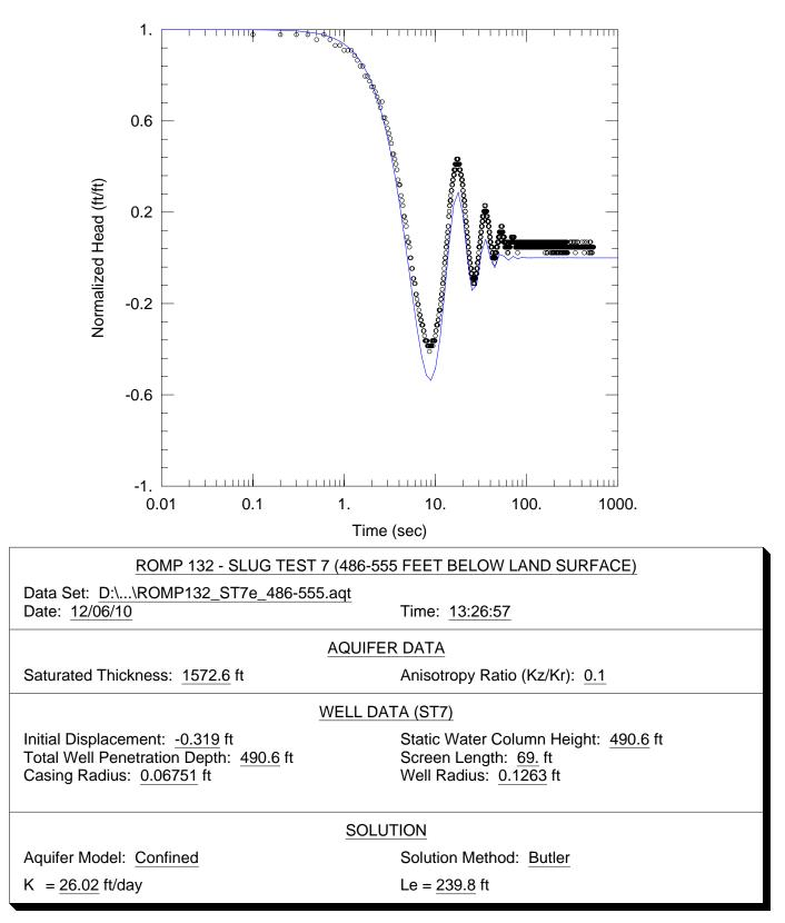
**Figure F-7.** Curve match solution from AQTESOLV<sup>®</sup> for hydraulic conductivity (K) using data from the slug test conducted between 486 and 555 feet below land surface (slug test 7) at the ROMP 132 well site in Marion County.
