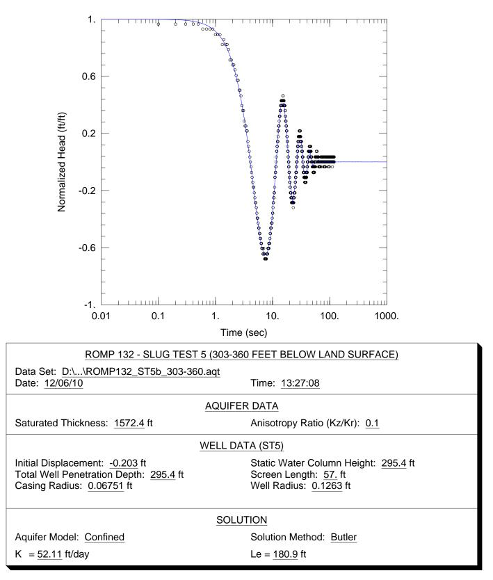
**Figure F-5.** Curve match solution from AQTESOLV<sup>®</sup> for hydraulic conductivity (K) using data from the slug test conducted between 303 and 360 feet below land surface (slug test 5) at the ROMP 132 well site in Marion County.
