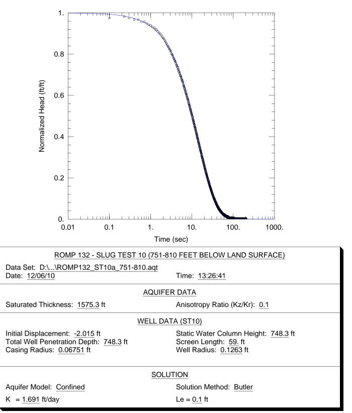
**Figure F-10.** Curve match solution from AQTESOLV<sup>®</sup> for hydraulic conductivity (K) using data from the slug test conducted between 751 and 810 feet below land surface (slug test 10) at the ROMP 132 well site in Marion County.
