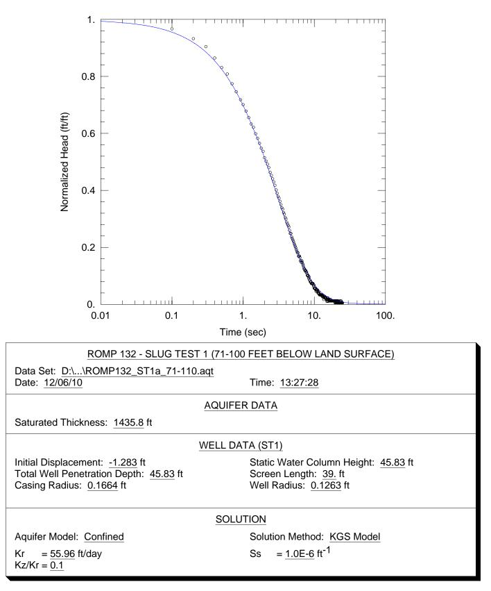
**Figure F-1.** Curve match solution from AQTESOLV<sup>®</sup> for hydraulic conductivity (Kr) using data from the slug test conducted between 71 and 110 feet below land surface (slug test 1) at the ROMP 132 well site in Marion County.
