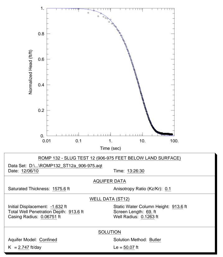
**Figure F-12.** Curve match solution from AQTESOLV<sup>®</sup> for hydraulic conductivity (K) using data from the slug test conducted between 906 and 975 feet below land surface (slug test 12) at the ROMP 132 well site in Marion County.
