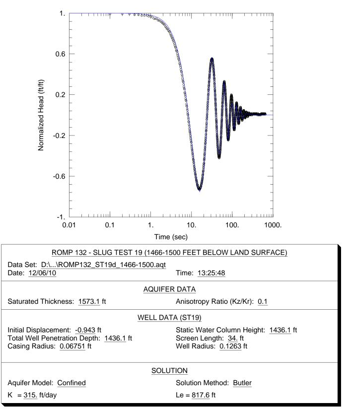
**Figure F-19.** Curve match solution from AQTESOLV<sup>®</sup> for hydraulic conductivity (K) using data from the slug test conducted between 1,466 and 1,500 feet below land surface (slug test 19) at the ROMP 132 well site in Marion County.
