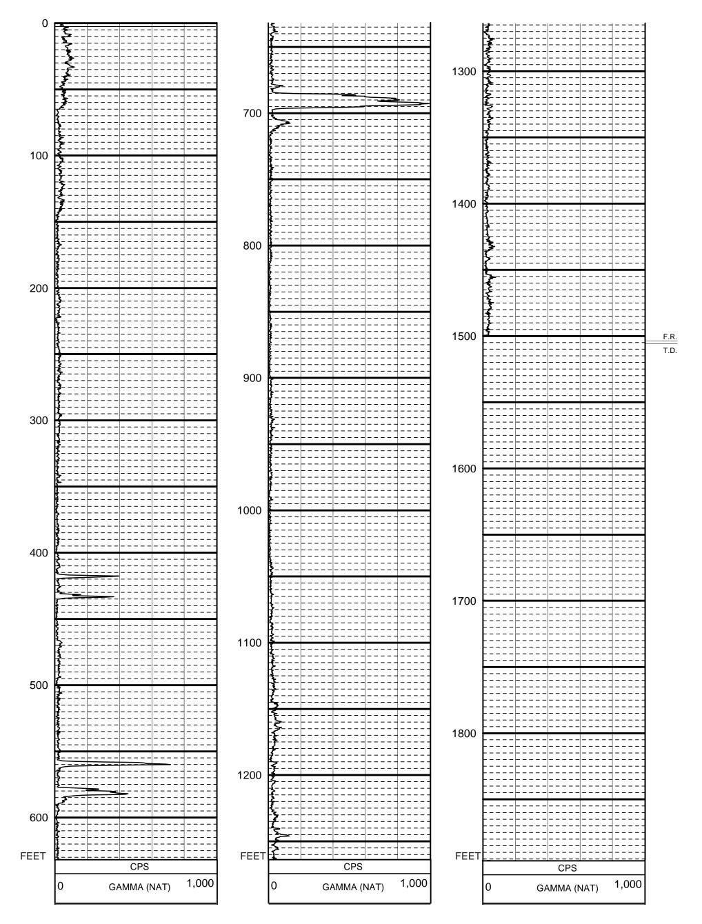
**Figure B-4.** Geophysical log collected in the exploratory core hole, between land surface and 1,505 feet below land surface, during exploratory coring at the ROMP 132 well site in Marion County, Florida. The logs were collected on 1/21/2009 using tool 9165C (caliper/gamma). The casing depth at the time of logging was 1,500 feet below land surface (see figure B-1). The vertical log scale is 2 inches per 100 feet.
