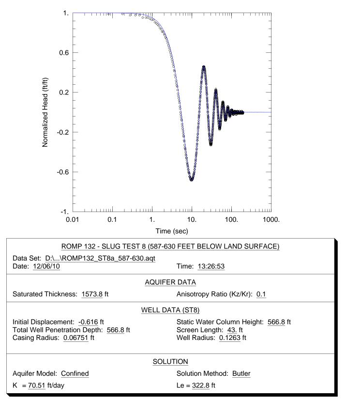
**Figure F-8.** Curve match solution from AQTESOLV<sup>®</sup> for hydraulic conductivity (K) using data from the slug test conducted between 587 and 630 feet below land surface (slug test 8) at the ROMP 132 well site in Marion County.
