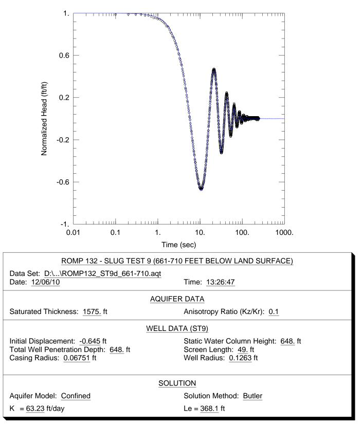
**Figure F-9.** Curve match solution from AQTESOLV<sup>®</sup> for hydraulic conductivity (K) using data from the slug test conducted between 661 and 710 feet below land surface (slug test 9) at the ROMP 132 well site in Marion County.
