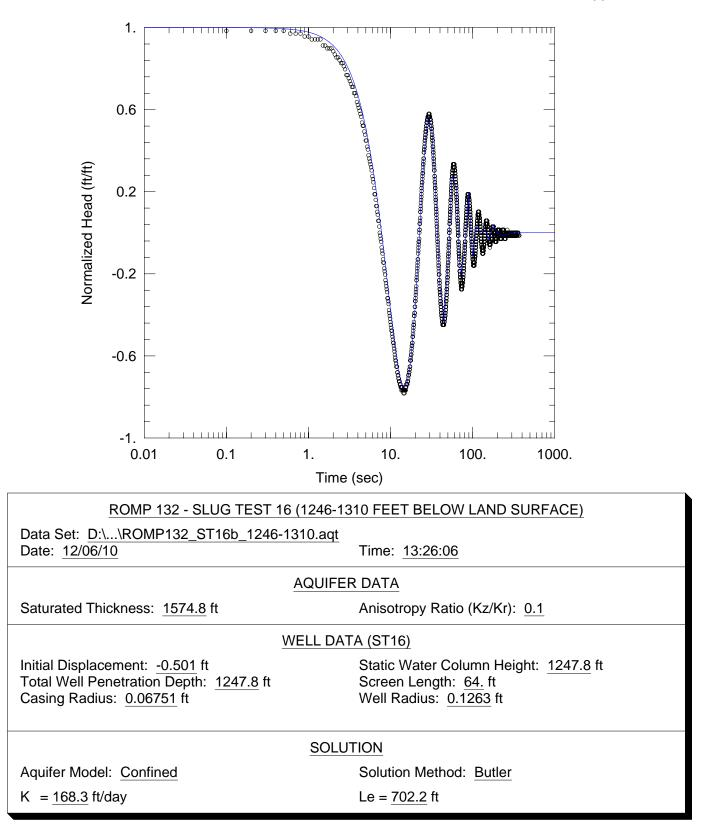
**Figure F-16.** Curve match solution from AQTESOLV<sup>®</sup> for hydraulic conductivity (K) using data from the slug test conducted between 1,246 and 1,310 feet below land surface (slug test 16) at the ROMP 132 well site in Marion County.
