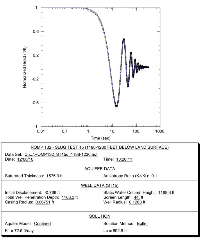
**Figure F-15.** Curve match solution from AQTESOLV<sup>®</sup> for hydraulic conductivity (K) using data from the slug test conducted between 1,186 and 1,230 feet below land surface (slug test 15) at the ROMP 132 well site in Marion County.
