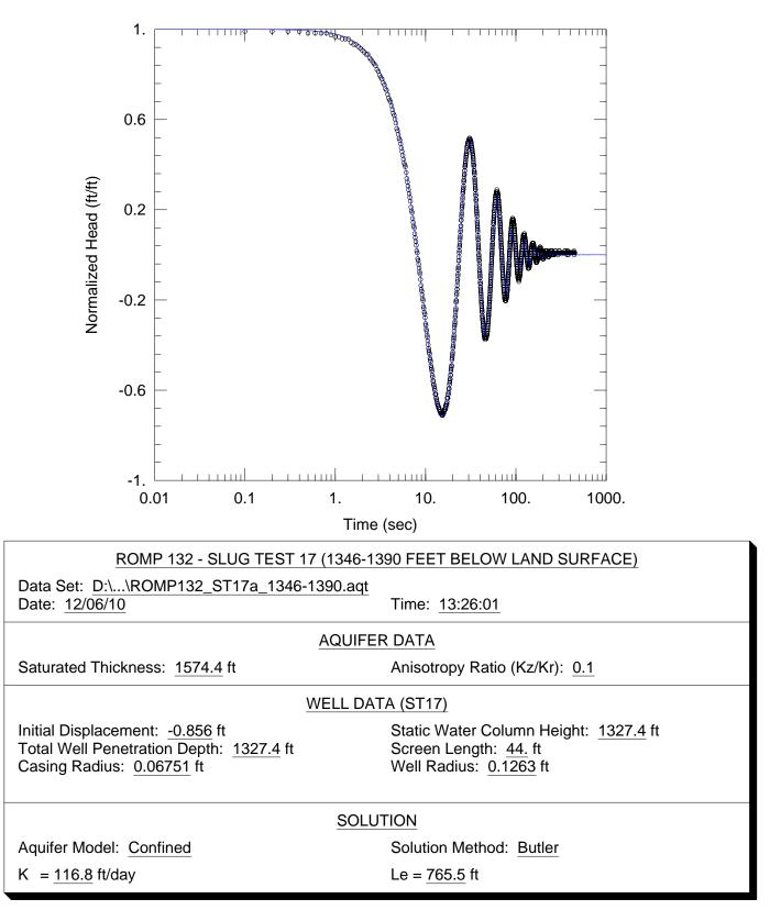
**Figure F-17.** Curve match solution from AQTESOLV<sup>®</sup> for hydraulic conductivity (K) using data from the slug test conducted between 1,346 and 1,390 feet below land surface (slug test 17) at the ROMP 132 well site in Marion County.
