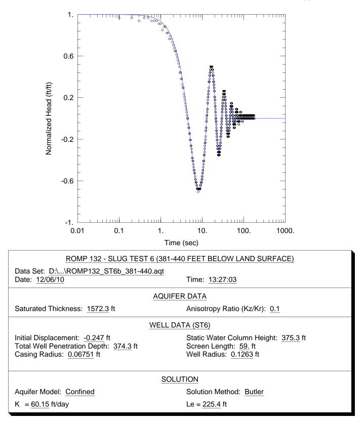
**Figure F-6.** Curve match solution from AQTESOLV<sup>®</sup> for hydraulic conductivity (K) using data from the slug test conducted between 381 and 440 feet below land surface (slug test 6) at the ROMP 132 well site in Marion County.
