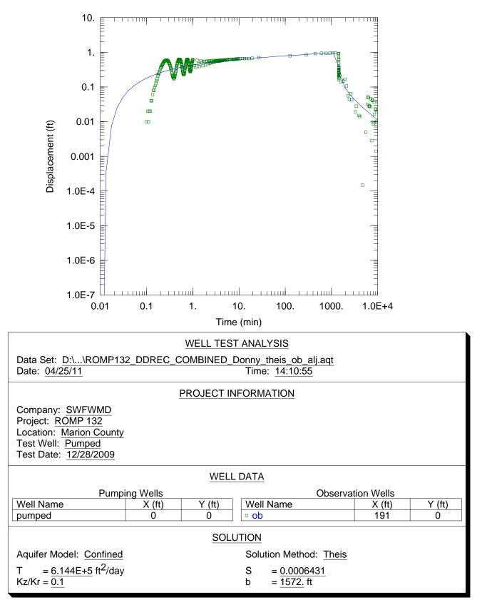
**Figure H-3.** Curve match solution output from AQTESOLV<sup>®</sup> using the Theis/Hantush method for the estimation of transmissivity (T) using groundwater level data collected from the Upper Floridan aquifer monitor well during the Upper Floridan aquifer performance test at the ROMP 132 well site in Marion County.
