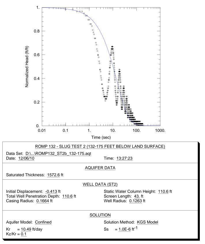
**Figure F-2.** Curve match solution from AQTESOLV<sup>®</sup> for hydraulic conductivity (Kr) using data from the slug test conducted between 132 and 175 feet below land surface (slug test 2) at the ROMP 132 well site in Marion County.
