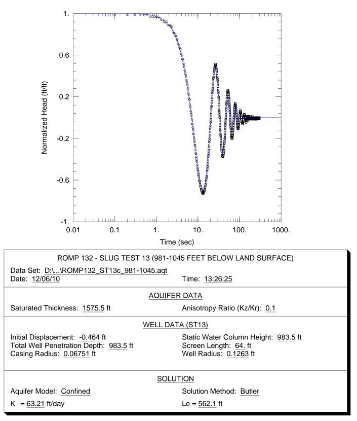
**Figure F-13.** Curve match solution from AQTESOLV<sup>®</sup> for hydraulic conductivity (K) using data from the slug test conducted between 981 and 1,045 feet below land surface (slug test 13) at the ROMP 132 well site in Marion County.
