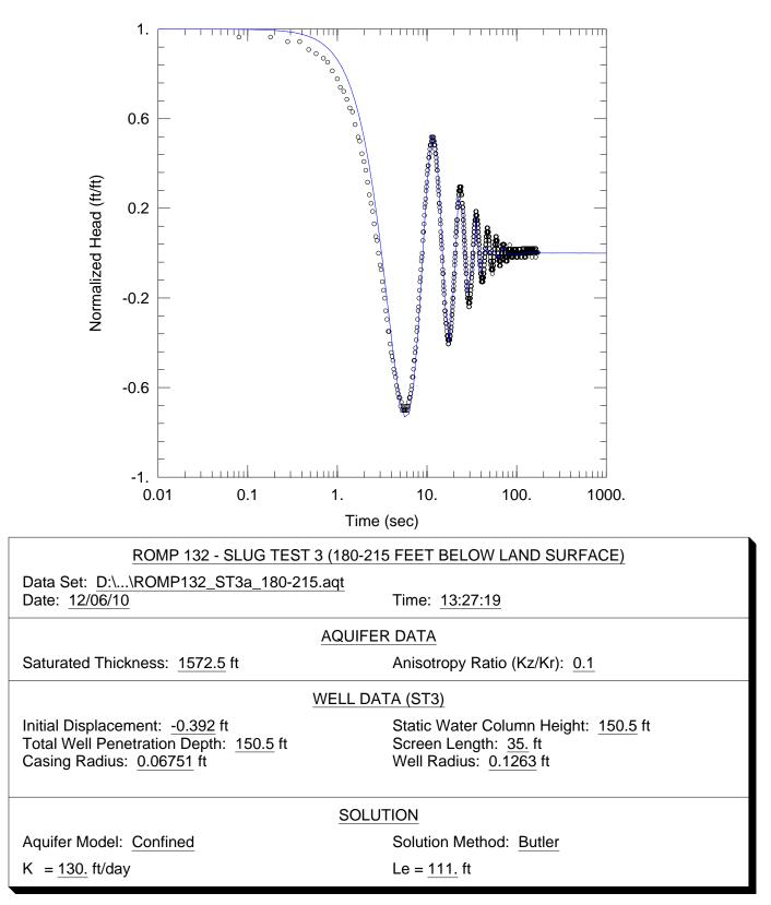
**Figure F-3.** Curve match solution from AQTESOLV<sup>®</sup> for hydraulic conductivity (K) using data from the slug test conducted between 180 and 215 feet below land surface (slug test 3) at the ROMP 132 well site in Marion County.
