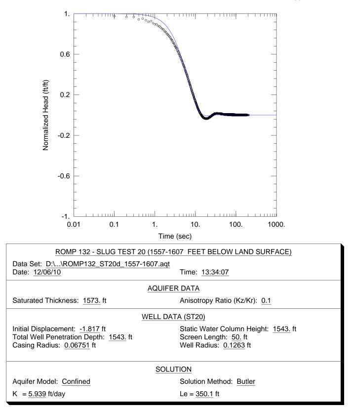
**Figure F-20.** Curve match solution from AQTESOLV<sup>®</sup> for hydraulic conductivity (K) using data from the slug test conducted between 1,557 and 1,607 feet below land surface (slug test 20) at the ROMP 132 well site in Marion County.
