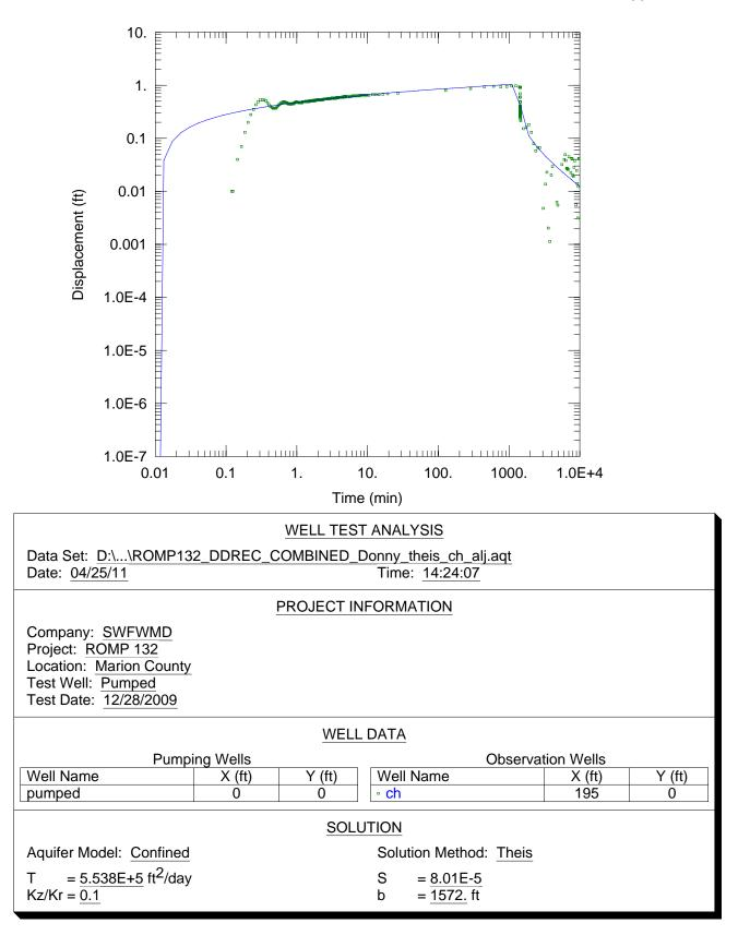
**Figure H-2.** Curve match solution output from AQTESOLV<sup>®</sup> using the Theis/Hantush method for the estimation of transmissivity (T) using groundwater level data collected from the exploratory core hole during the Upper Floridan aquifer performance test at the ROMP 132 well site in Marion County.
