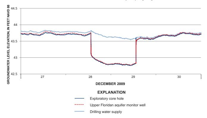
**Figure 7.** Hydrograph of groundwater levels in three wells before, during, and after the Upper Floridan aquifer performance test at the ROMP 132 well site in Marion County, Florida.
