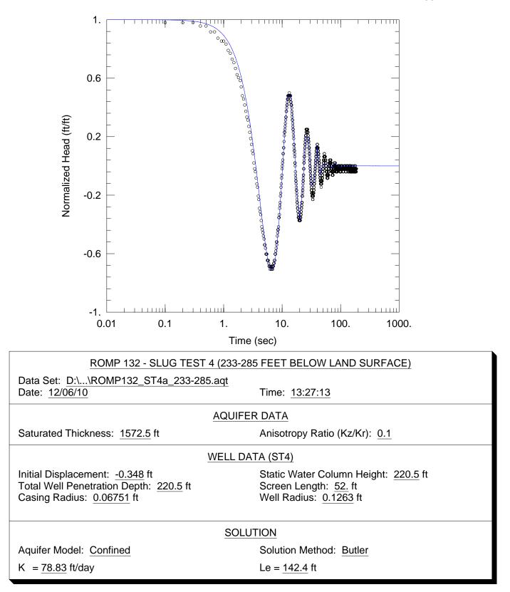
**Figure F-4.** Curve match solution from AQTESOLV<sup>®</sup> for hydraulic conductivity (K) using data from the slug test conducted between 233 and 285 feet below land surface (slug test 4) at the ROMP 132 well site in Marion County.
