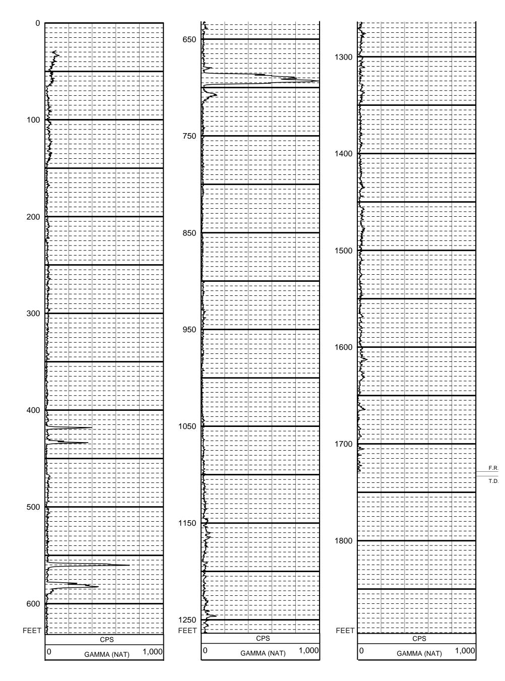
**Figure B-5.** Geophysical log collected in the exploratory core hole, between land surface and 1,734 feet below land surface, during exploratory coring at the ROMP 132 well site in Marion County, Florida. The logs were collected on 9/15/2010 using tool 9165C (caliper/gamma). The casing depth at the time of logging was 1,734 feet below land surface (see figure B-1). The vertical log scale is 2 inches per 100 feet.
