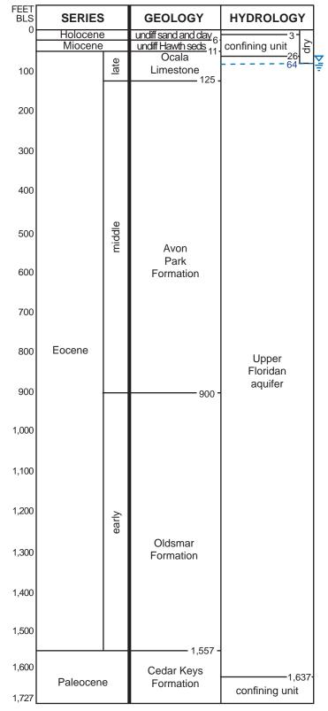
[Not to scale; Land surface elevation = 108 feet above the North American Vertical Datum of 1988; bls, below land surface; undiff, undifferentiated; undiff Hawth seds, undifferentiated Hawthorn Group sediments]
