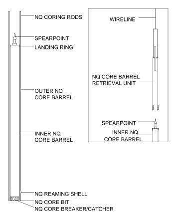
**Figure A-1.** Boart Longyear<sup>®</sup> NQ Wireline Coring Apparatus.
