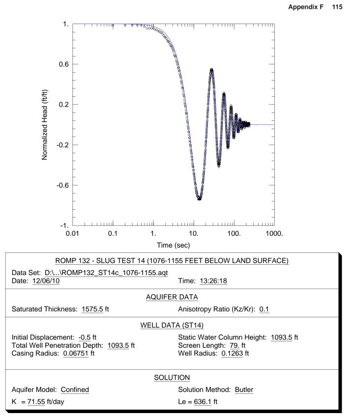
Figure F-14. Curve match solution from AQTESOLV® for hydraulic conductivity (K) using data from the slug test conducted between 1,076 and 1,155 feet below land surface (slug test 14) at the ROMP 132 well site in Marion County.
