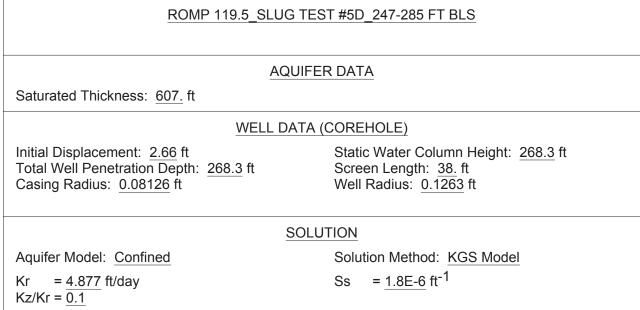
**Figure G4.** Curve-match analysis for slug test #5D performed in core hole 1 at the ROMP 119.5 well site in Marion County, Florida.
