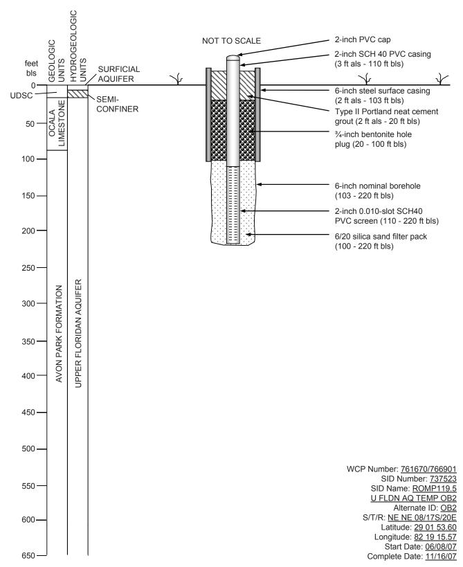
**Figure B10.** Well as-built diagram for the Upper Floridan aquifer temporary observation well (OB2) at the ROMP 119.5 well site in Marion County, Florida.
