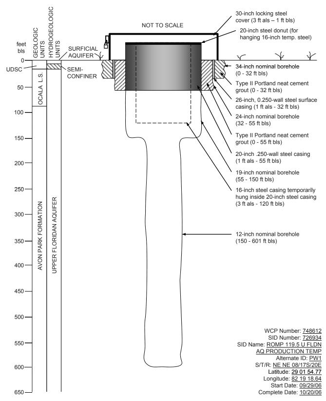
**Figure B8.** Well as-built diagram for the Upper Floridan aquifer temporary production well at the ROMP 119.5 well site in Marion County, Florida.
